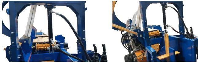
Install the Log Stop. Log Stop openings downwards.
