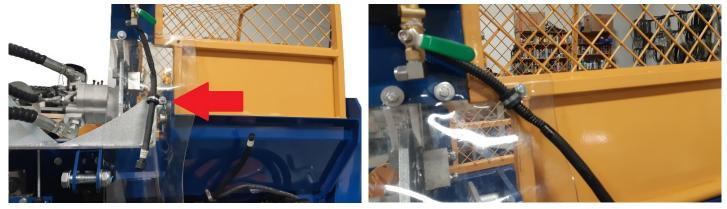
Tighten the valve for the saw oil. Then install the hose.
