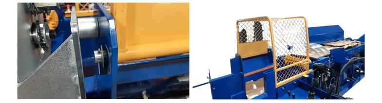
Remove all bolts on the cage. Lift the saw cover onto the machine and install all bolts.
