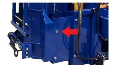
Raise the infeed table until the legs are in the air. Take the 4 bolts out on both legs. Take off the stands.
