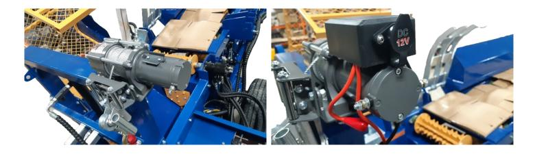
Connect the cables to the winch motor. Red to plus and black to minus.
