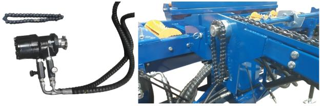
The sprocket may need to be adjusted. So that the chain can run freely without rubbing.
