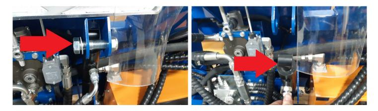
Insert the cylinder into the bracket and install the bolt.
