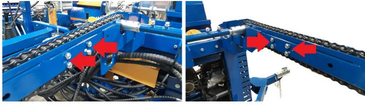
Install the inner crossbar. Bracket for the hydraulic cylinder downwards.
