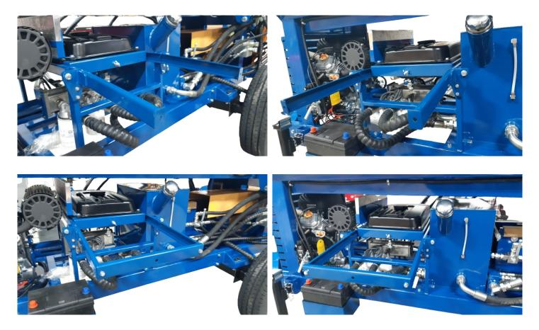
Now remove the wing nut on the other side of the tank. Pull the tank slightly out onto the rails. This aligns the rails. Now tighten all bolts. If the tank does not slide easily, readjust the rails. Push back the tank and reinstall the wing nut on the other side of the tank.
