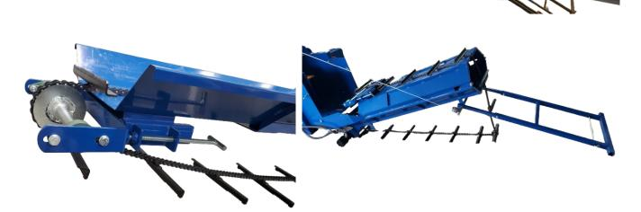
Pull the chain inside the machine towards the splitter wedge. Lift the conveyor until upright.
