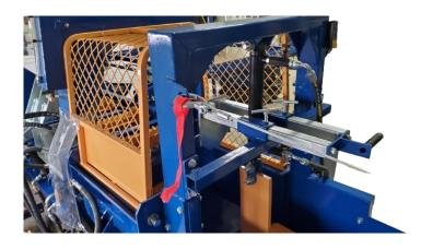
Roll in the cable with the winch. Watch the cable is correct on the rollers. Close the safety latch and install the safety pin underneath the conveyor.
