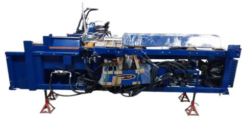
Cut the straps holding the panel and remove the panel from the machine.
