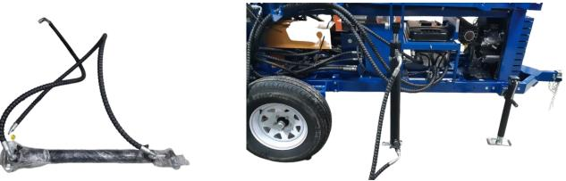
Install the cylinder at the bottom of the frame.
