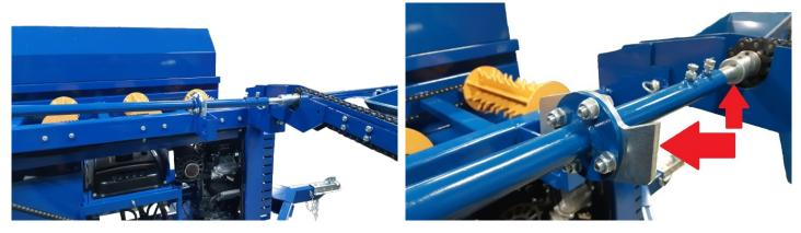
Remove the bushing on the other side. Install on the chain shaft as in the picture.
