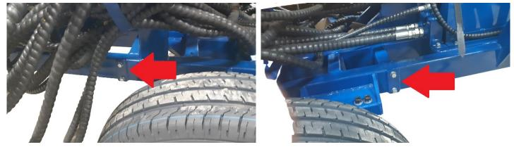
First install the bars for the fender. Bolt them to the frame. Then bolt the fender onto these.
