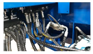
There is a smaller hose connected to the regeneration valve which is not yet connected at the other end. This must be connected to one of the two hydraulic pressure gauge. There is a very small seal in this hose connection. Check that this seal is present.
