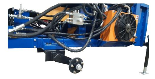
Install the wheels. Torque to 80 fb/lbs. Check the tire pressure according to the manufacturer's value on the tire.
