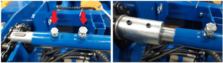
Insert the key and push the rod as far as it will go into the bushing.
