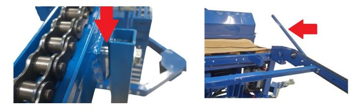
Now install the hydraulic motor. Hang the chain over the upper sprocket.
