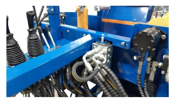
A further hose is connected under the Panel on one side only. The picture shows which hose this is. This hose will be connected to the valve for the log table.
