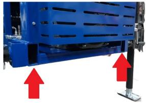
Install the tow bar and tighten all bolts.
