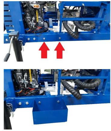
These parts make up the fuel tank slide. Install as shown in the pictures. The arrows show where the parts are installed on the frame. Leave all bolts loose for now.
