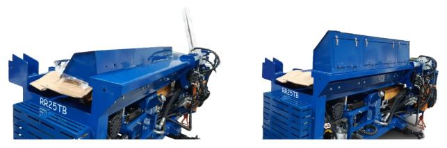
The next step is to attach the tow bar. To do this, these two adapters must first be inserted into the frame and the bolts installed. Leave the bolts loose.
