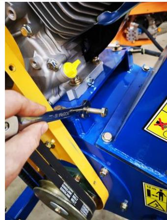
Now tighten the 4-16mm bolts holding the engine plate
