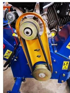
Re-install the 4-13mm bolts in the belt cover
