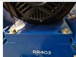
Re-install the 2-13mm bolts in the inner belt cover, center the cover over the pulleys and tighten the bolts
