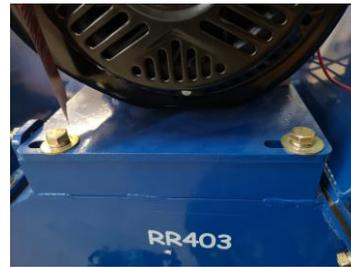
Tighten the belt adjustment bolts. Adjust each bolt  $\frac{1}{4}$  turn at a time until you have less than 1" of deflection on the belts.
