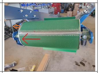
Double check the lower roller, adjust if needed.
