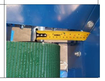
Now measure from the centre of the shaft on the bearing side to the edge of the frame.
