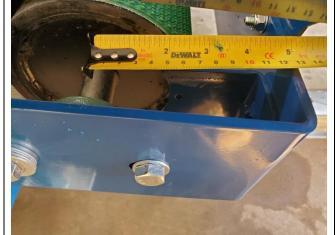
Use the adjuster bolt to make the measurement the same on both sides. Now the bottom roller should be square.
