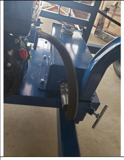
Install the pressure hose from the pump to the control valve,
