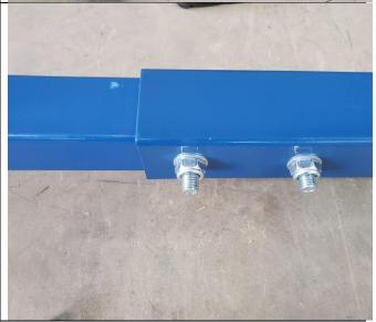
The 2 longer conveyor sections will have flanges that bolt together, remove the 7 - 16mm bolts  $\times$  17mm nuts,
