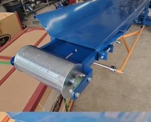
Tighten the 10mm nut and bolt, leave it loose enough that the roller can still slide when adjusting it.
