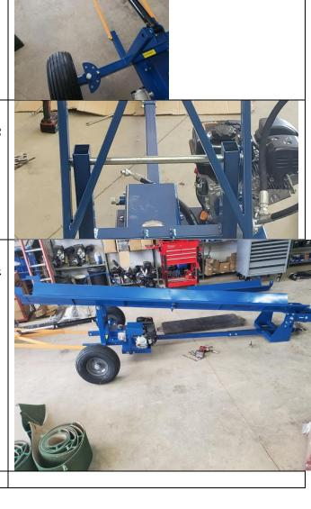
On the lower end, loosen the bearing set screws, move the pins until they line up with the frame holes and insert the pin.
