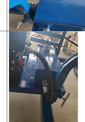
Install the pressure hose from the pump to the control valve,
