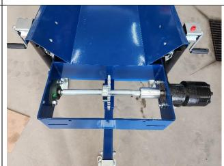
Insert the control valve arm and tighten the T-Handle.
