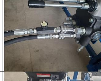
Install the suction hose between the tank and pump.
