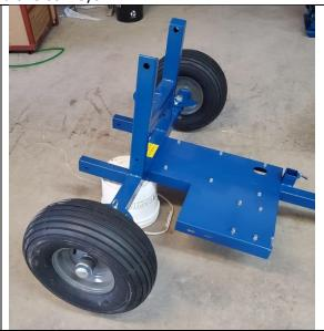
Remove the 4 - 13mm nuts from the engine mount studs, place the engine with the hydraulic pump positioned towards the wheels, close to the hydraulic filler cap. Push the studs up from the bottom through the holes in the base of the engine and attach the 13mm nuts.
