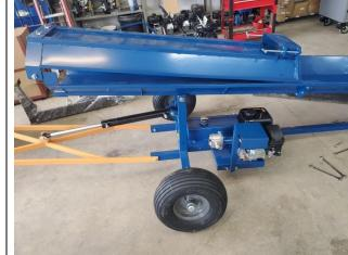
Insert the bolts with the nuts on the outside and tighten, leave some looseness so the sections can swivel.
