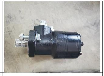
Tighten the 16mm Bolt  $\,\times\,$  17mm nut, tighten both allan keys on the coupler.
