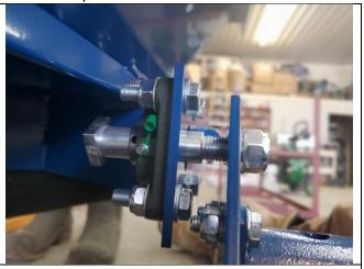
Set the last conveyor trough section in place, upside down.
