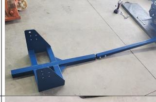
Remove the 2 - 16mm bolts  $\times$  17mm nuts, line up the holes in the 2 frame sections, reinstall the 2 bolts and nuts and tighten.
