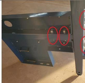
Tighten the swivel bolt until there is no up and down movement in the axle stub, but the axle stub must be able to move freely from side to side.
