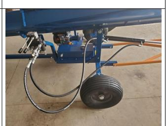
The needle valve is used to control the speed that the conveyor goes up, it is best to start with the needle valve mostly closed and then adjust to your desired speed once you have the conveyor running.
