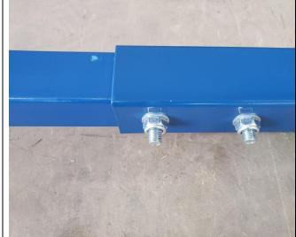
The 2 longer conveyor sections will have flanges that bolt together, remove the 7 - 16mm bolts  $\times$  17mm nuts,
