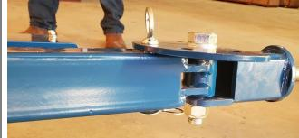
Mount the tires onto the stub axle and tighten the nut until you can insert the cotter pin into the castle nut.
