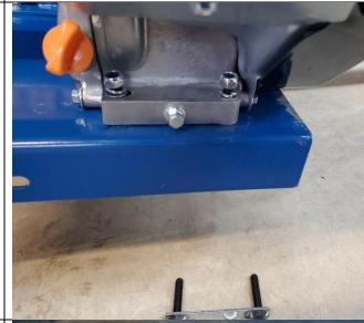
Once all 4 - 13mm nuts are threaded on, tighten them securing the engine into place.
