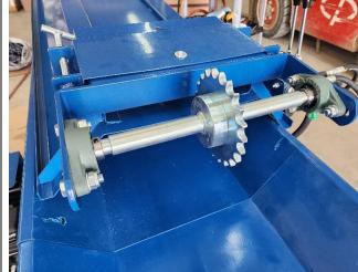
Tighten the 10mm nut and bolt, leave it loose enough that the roller can still slide when adjusting it.
