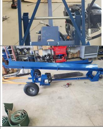
On the lower end, loosen the bearing set screws, move the pins until they line up with the frame holes and insert the pin.
