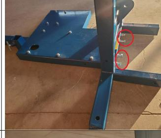
Lift the frame up and insert the 2 -16mm bolts with the 17mm nuts, tighten these and then tighten the 4 - 16mm bolts in the red circle as well.
