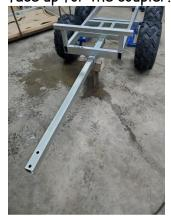
9.) Large bolt goes through frame tube and main frame, tighten nut. Tighten 2 bolts on the side of the frame rail, then tighten retaining nuts.
