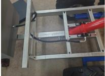
15.) Run the hydraulic hose trough the clips and bend the clips to hold the hose in place. Use zip ties to secure the hose in place.
