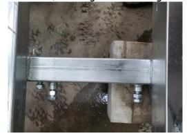
10.) Slide battery box onto frame tube and then slide the tongue jack on, install the 2 retainer bolts for the battery box but do not tighten, Move the tongue jack approximately 12cm back from coupler bolt hole and tighten the retainer bolt. (note battery box may be grey, blue or black)
