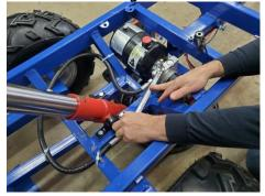
8) Re-install solenoid and tighten nut by hand only.
