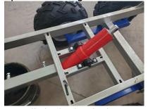
14.) <u>Install the hydraulic hose onto</u> the cylinder and tighten.
