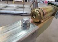
13.) Install hydraulic fitting into cylinder (if not pre-Installed), install brackets and cylinder on frame, hydraulic fitting should be facing the side with the hose retainer straps, tighten all 4 bolts.
