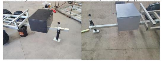
11.) Slide the swivel coupler mount in, position the swivel up or down depending on your ATV hitch height, tighten both bolts.
