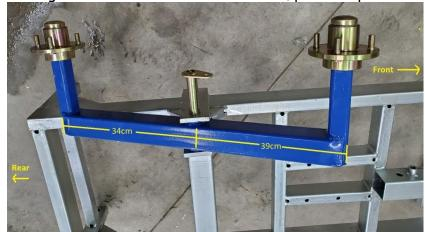
4.) Install 13mm bolt & nut washer through the plate on the pin and the frame tab, tighten nut & bolt. Install cotter pin, repeat for the opposite side.
