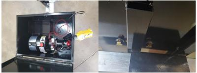
17.) Atatch the hose to the hydraulic pump.
