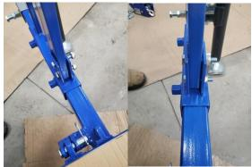
13.) Mount winch and tighten nuts.
