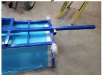
5.) Use bolts with the spacers to bolt the tongue frame tube to the subframe, tighten bolts.
