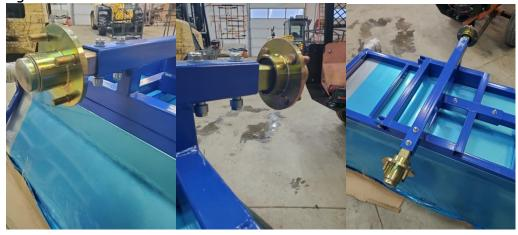
8.) Install all 4 tires and tighten wheel nuts to 40ft/lbs.
