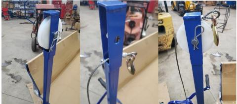
16.) Attach winch hook to loop on the front of the tub, please remember the retaining pin must be removed before the tub can be winch up into the air.
