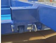
7.) Insert the axle tubes into the subframe and use bolts with spacers in the 2 holes provided, tighten the bolts.
