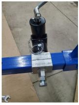
20.) Install swivel hitch and tighten the bolts.
