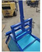
6.) Insert pin to hold the front of the tub to the trailer frame and use "R" clip to retain pin.
