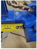
18.) <u>Tighten the retaining bolts in the winch mount and then tighten the retaining nuts.</u>
