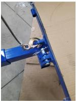
17.) Slide the winch mount support to be 6-7 cm away from the support pin tube, any closer and the winch handle may touch the front tub door.
