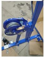
14.) Attach winch handle and tighten.
