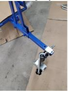
12.) Mount the winch cable support but to the winch mount, tighten bolts but leave room for the bar to have some movement.
